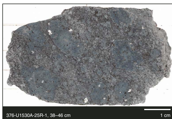
Figure F20. A–C. Alteration Subtype IIIb, Hole U1530A. Illite-smectite (smec) matrix with intergrowth of quartz (Qtz) and disseminated pyrite locally oxidized to \text{FeO}(\text{OH}) .
