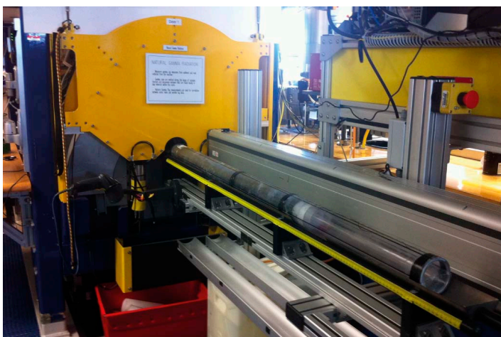
Figure F10. Natural Gamma Radiation Logger for whole-round cores. It conducts 8 measurements at a time in 2 positions, resulting in 16 measurements per core when measuring at both positions.
