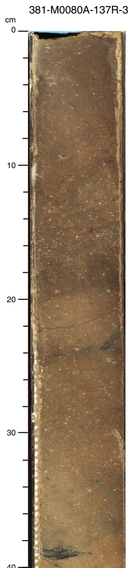
Figure F16. Typical FA16 (greenish to buff bedded and bioturbated bioclastic sandstone to mudstone) showing faintly bedded brown grayish very fine sandstone with abundant ostracods and other shell fragments, Hole M0080A Subunit 4-2. Top of core image is at 503.24 mbsf.
