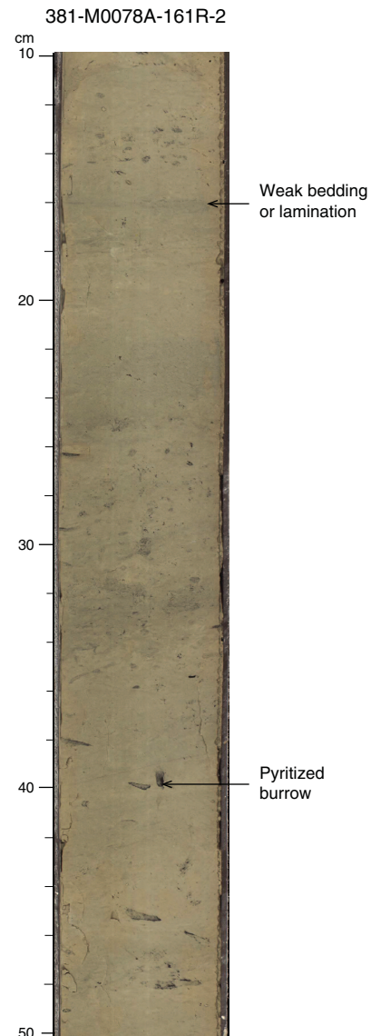
Figure F12. Typical section of FA12 (light gray to buff homogeneous to weakly stratified bioturbated mud) showing pale gray heavily bioturbated homogeneous mud, Hole M0078A Unit 2. Faint laminations and abundant organic flecks can be seen throughout the section; a pyritized burrow is also shown. Top of core image is at 549.55 mbsf.
