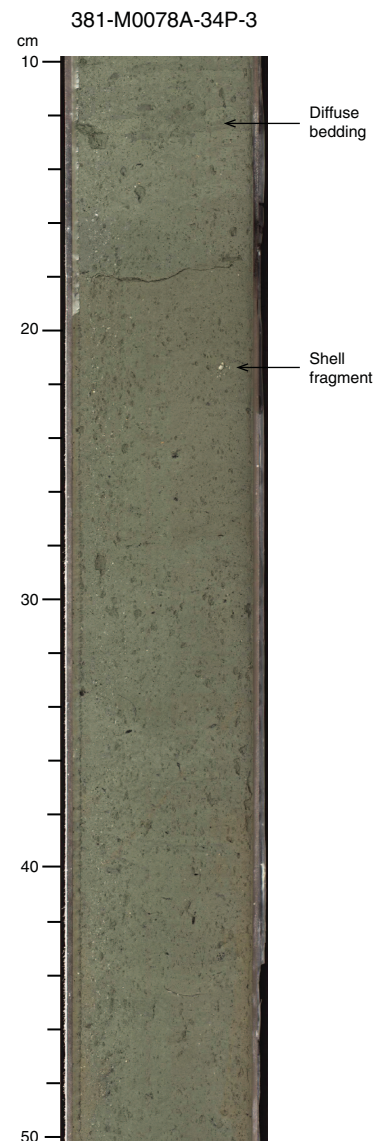
Figure F1. FA1 (homogeneous mud) consists of greenish gray homogeneous mud with diffuse bedding and scattered shell fragments, Hole M0078A Sub-unit 1-3. Top of core image is at 97.00 mbsf.
