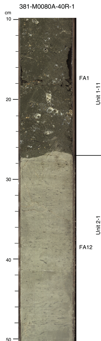
Figure F7. Erosive boundary between Units 1 and 2 at 27 cm (136.96 mbsf), Hole M0080A. Boundary separates FA1 greenish gray mud in Unit 1 (above) from FA12 white/light gray bioturbated mud in Unit 2 (below). Top of core image is at 136.80 mbsf.
