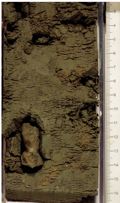
Figure F6. Part of lithified burrow (382-U1534A-22F-CC, 11–15 cm).
