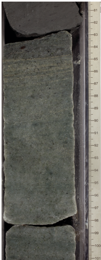
Figure F8. Part of 34 cm long greenish gray, graded glauconite containing quartz sandstone with silt laminations (382-U1536E-18R-1, 81–101 cm).
