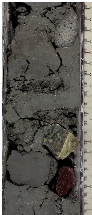
Figure F10. Example of dropstone-rich interval containing three types of igneous rocks (382-U1536E-21R-1, 19–37 cm). Interval is near top of first section, so dropstones are not in place (fall-in).
