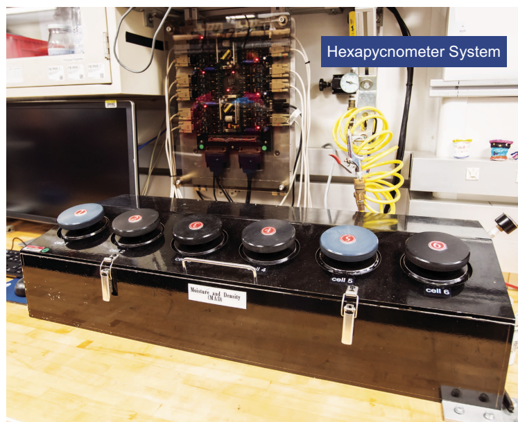
Figure F30. Hexapycnometer system for volume measurements.
