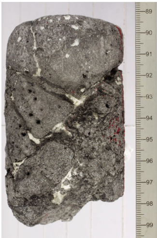
Figure F25. Fault plane displacing small blocks and truncating their bounding fractures in a zone of internal brecciation in hypabyssal igneous rock (385-U1547D-19R-1, 89–100 cm). White vein-filling material (mainly carbonate) is distributed irregularly along the fault and at the intersections with the truncated fractures, indicating that it filled the fractures after slip had taken place on them.
