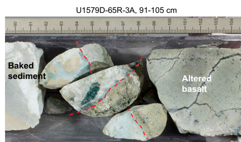
Figure F14. Partial recovery of Lithostratigraphic Unit V (sediment)/VI (basalt) contact (392-U1579D-65R-3, 91–105 cm). The basalt is completely altered, and the sediment shows signs of contact metamorphism. The contact (red dashed line) was not recovered oriented, so individual pieces were arranged to better show the contact.
