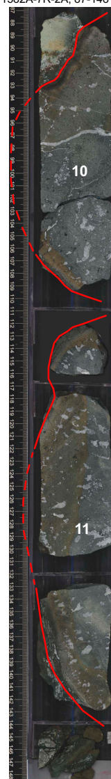
Figure F10. Two pillow lava lobes (Igneous Units 10 and 11; 392-U1582A-7R-2). Solid red lines = curved chilled margins, dashed red lines = extrapolation of the margins. The rocks of Igneous Unit 11 show radial bands of vesicles trains (filled with white carbonate), which are typical for pillow lava lobes. Note the broad reddish brown oxidation halo running subparallel inward of the margins. A small piece of green carbonate sediment, visible at the top left of Igneous Unit 10, represents interpillow sediment.
