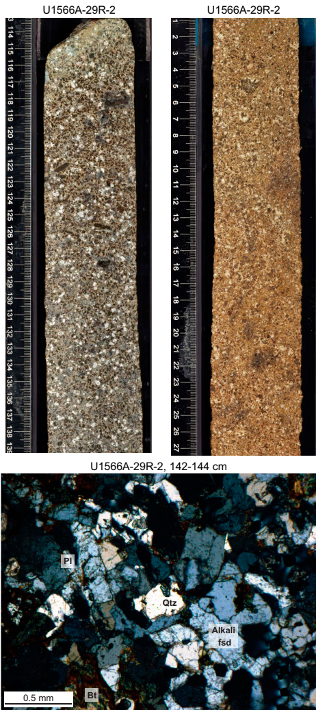
Figure F11. Granite, Hole U1566A. Top: comparison between weakly altered granite with biotite (left) and decomposed granite (right). Bottom: weakly altered granite showing its main mineralogy (XPL). Pl = plagioclase, bt = biotite, qtz = quartz, fsd = feldspar.
