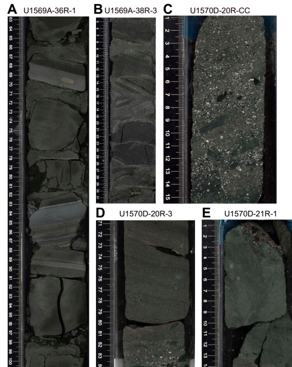
Figure F10. Lithologic characteristics of Units VII and VIII, Holes U1569A and U1570D. A. Very dark gray ash-rich siltstone with clay and diagenetic pyrite (Unit VII). B. Ash layers showing parallel lamination (Unit VII). C. Dark green tuffaceous siltstone. D. Color change from dark gray to dark green siltstone transitioning to tuffaceous siltstone in Unit II. A fragment of wood is observed in this interval. E. Unit VII–VIII transition, Hole U1570D. Transition is marked by an erosional surface that separates the tuffaceous siltstone observed in Section 20R-CC from the dark greenish gray bioturbated siltstone with clay that characterizes Unit VIII.
