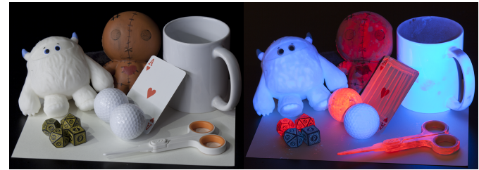
Fig. 3. Objects covered with our fluorescent ink (UV-blue and UV-red). (left) Image under visible light. (right) Image under UV light, where the fluorescent colors become visible.
