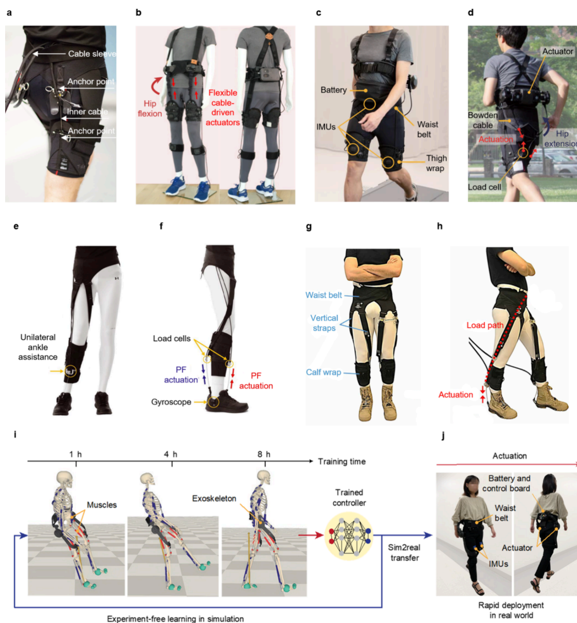
Figure 9. Lower body soft wearable robots. (a) Photograph of a hip soft exosuit that can reduce the energy expenditure of walking, actuated by inner cable. Reproduced with permission from ref 262. Copyright 2018 The American Association for the Advancement of Science. (b) Components of the soft robotic apparel with cable-driven actuators and sensors for hip flexion assistance to avert freezing of gait in Parkinson's disease. Reproduced with permission from ref 263. Copyright 2024 Springer Nature. (c,d) Front (c) and back (d) views of a soft exosuit that reduces the metabolic rate for both running and walking via the hip extension. Reproduced with permission from ref 264. Copyright 2019 The American Association for the Advancement of Science. (e,f) Front (e) and side (f) views of a soft wearable robot with Bowden cable-based mechanical power transmissions to generate assistive joint torques, designed to augment paretic limb function during hemiparetic walking. Reproduced with permission from ref 265. Copyright 2017 The American Association for the Advancement of Science. (g,h) Front (g) and side (h) views of a tethered soft exosuit for metabolic cost reduction. Reproduced with permission from ref 266. Copyright 2017 The American Association for the Advancement of Science. (i,j) Neural networks-based controller training in simulation (i) and real-world deployment of an untethered exoskeleton without further training (j). Reproduced with permission from ref 267. Copyright 2024 Springer Nature.
