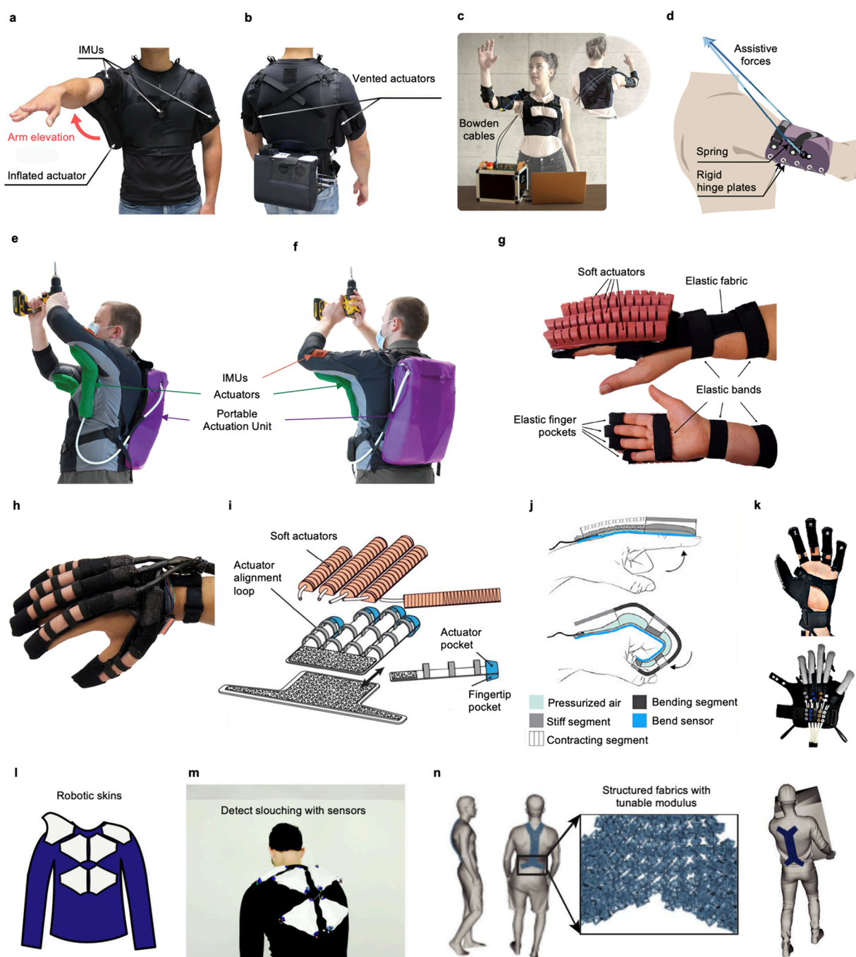
Figure 8. Upper body soft wearable robots. (a,b) Front (a) and back (b) views of an untethered, portable soft robotic wearable for restoring arm function. Reproduced with permission from ref 245. Copyright 2023 The American Association for the Advancement of Science. (c,d) Photograph (c) and schematic (d) of a textile exomuscle that supports the shoulder against gravity, with two Bowden cables highlighted in blue. Reproduced with permission from ref 248. Copyright 2022 Springer Nature. (e,f) Side (e) and back (f) views of an inflatable shoulder wearable robot to assist the shoulder during industrial work. Reproduced with permission from ref 249. Copyright 2024 The American Association for the Advancement of Science. (g) Top and bottom views of a soft pneumatic glove for hand rehabilitation. Reproduced with permission from ref 250. Copyright 2021 AIP Publishing. (h,i) Photograph (h) and exploded view (i) of a soft robotic glove with soft hydraulic actuators for combined assistance and at-home rehabilitation. Reproduced with permission from ref 251. Copyright 2015 Elsevier. (j,k) Schematic (j) and photographs (k) of a 2-DOFs inflatable soft glove with soft pneumatic actuators for improving motor function after stroke. Reproduced with permission from ref 252 under CC BY 4.0. Copyright 2024 Cambridge University Press. (l,m) Schematic (l) and photograph (m) of a modular, 2D soft robotic robot that can be reconfigured on the surface of passive, deformable bodies to produce deformations. Robotic skins attached to a garment detect poor posture and pulse to communicate with the wearer. Reproduced with permission from ref 253. Copyright 2018 The American Association for the Advancement of Science. (n) Reconfigurable fabrics for wearable medical supports (left) and exoskeletons (right). Reproduced with permission from ref 254. Copyright 2021 Springer Nature.
