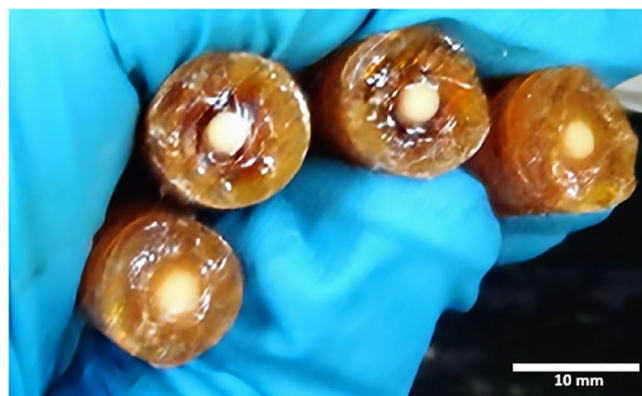
FIGURE 6 | Image of the cross section of the polymerized gels. Notice the difference in the middle vs. the outer layers.
