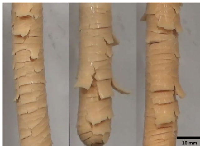
FIGURE 7 | Peeling observed from different positions around the same polymerized sample, with MHQ as the inhibitor.
