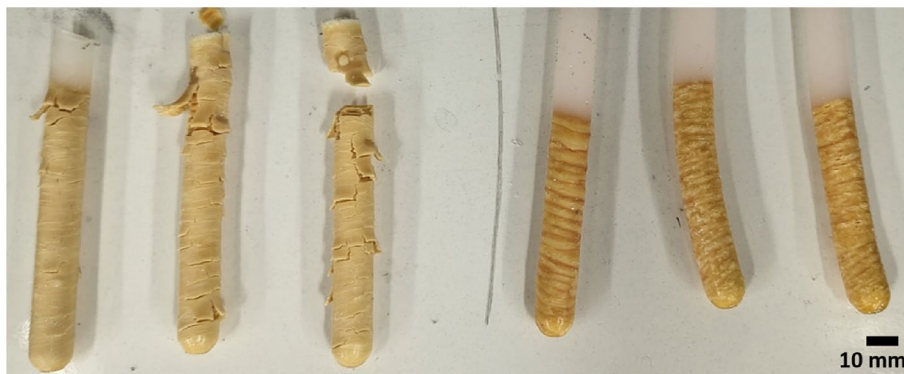
FIGURE 9 | Sample polymerized with no phenothiazine (left) vs. those with 0.5 phr phenothiazine (right). (TMPTA used in all samples contained about 250 ppm of MEHQ from the manufacturer). Notice that peeling is not observed in the samples containing phenothiazine.
