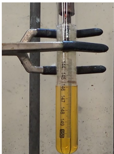
FIGURE 3 Charge transfer complex formation indicated by the appearance of yellow color and polymer formation indicated by the disappearance of yellow color into a 16 × 150 mm glass tube. The cured material is in the upper section.
