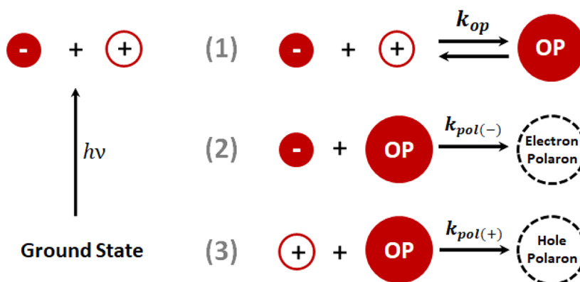
Figure 6. Pictorial representation of the rate processes in polaron formation whereby photoexcitation from the ground state produces free electrons and holes that generate optical phonons (1). These then couple to free electrons (2) and hole (3) to form electron and hole polarons, respectively.
