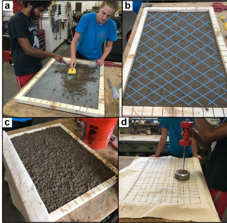
Figure 2. The synthetic bank construction process. (a) A fine layer of the bank mixture is pressed into a metal mesh. (b) The surface is scored in a cross-hatch pattern. (c) One third of the remaining mix is added. (d) The bank mix is uniformly compacted with modified 4.5 kg slide hammer. Steps b-d are repeated twice more.
