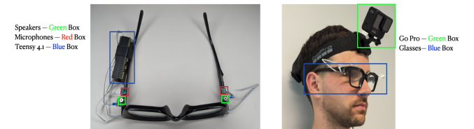
Figure 1: Glasses and GoPro Hardware setup for EchoGuide
