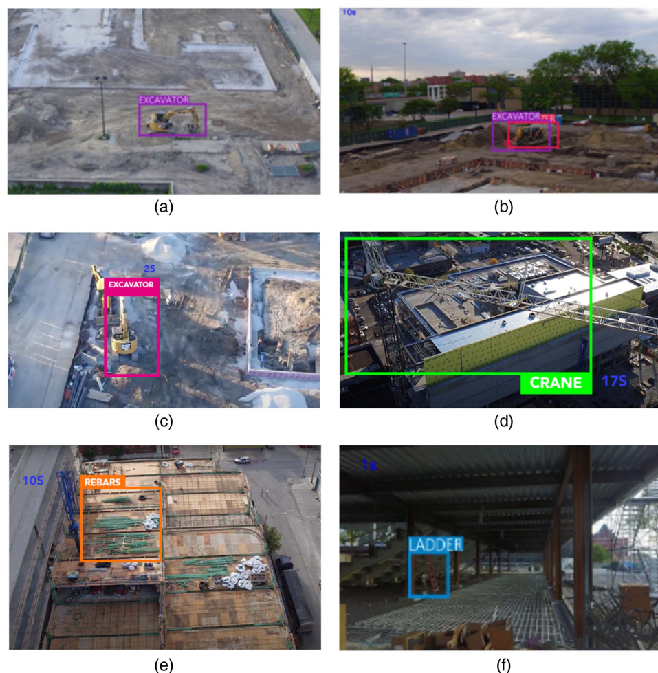
Fig. 7. Detected construction resources (classes) using predictors of the SSD models and UAV aerial images in real time: (a) excavator; (b) excavator and bulldozer; (c) excavator; (d) crane; (e) rebars; and (f) ladder. (Images by authors.)
