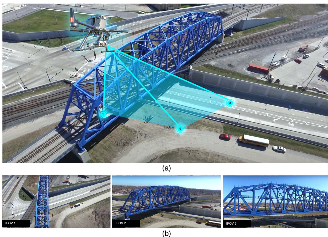
Fig. 2. Spatial and temporal resolutions: (a) shifting UAV motion and position in the construction zone airspace; and (b) IFOVs with different angle viewing, object sample sizes, and densities. (Image of UAV device and UAV images by authors.)
