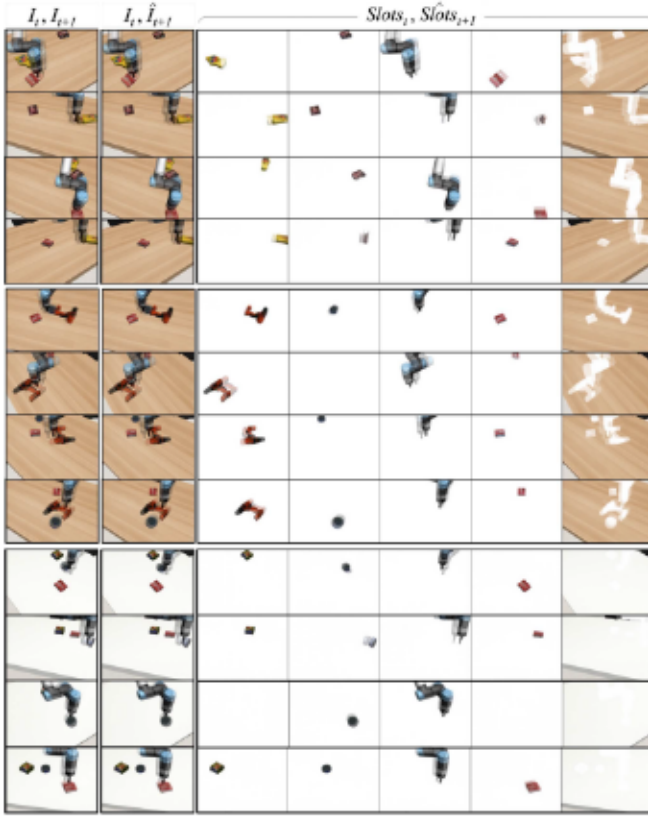
Fig. 10. Examples of single-step dynamics prediction using InvSlotGNN. Given the current scene image from an arbitrary uncalibrated camera angle, our model accurately predicts the future state of each slot based on the robot's pushing action in the world coordinate, and synthesizes the future scene image.
