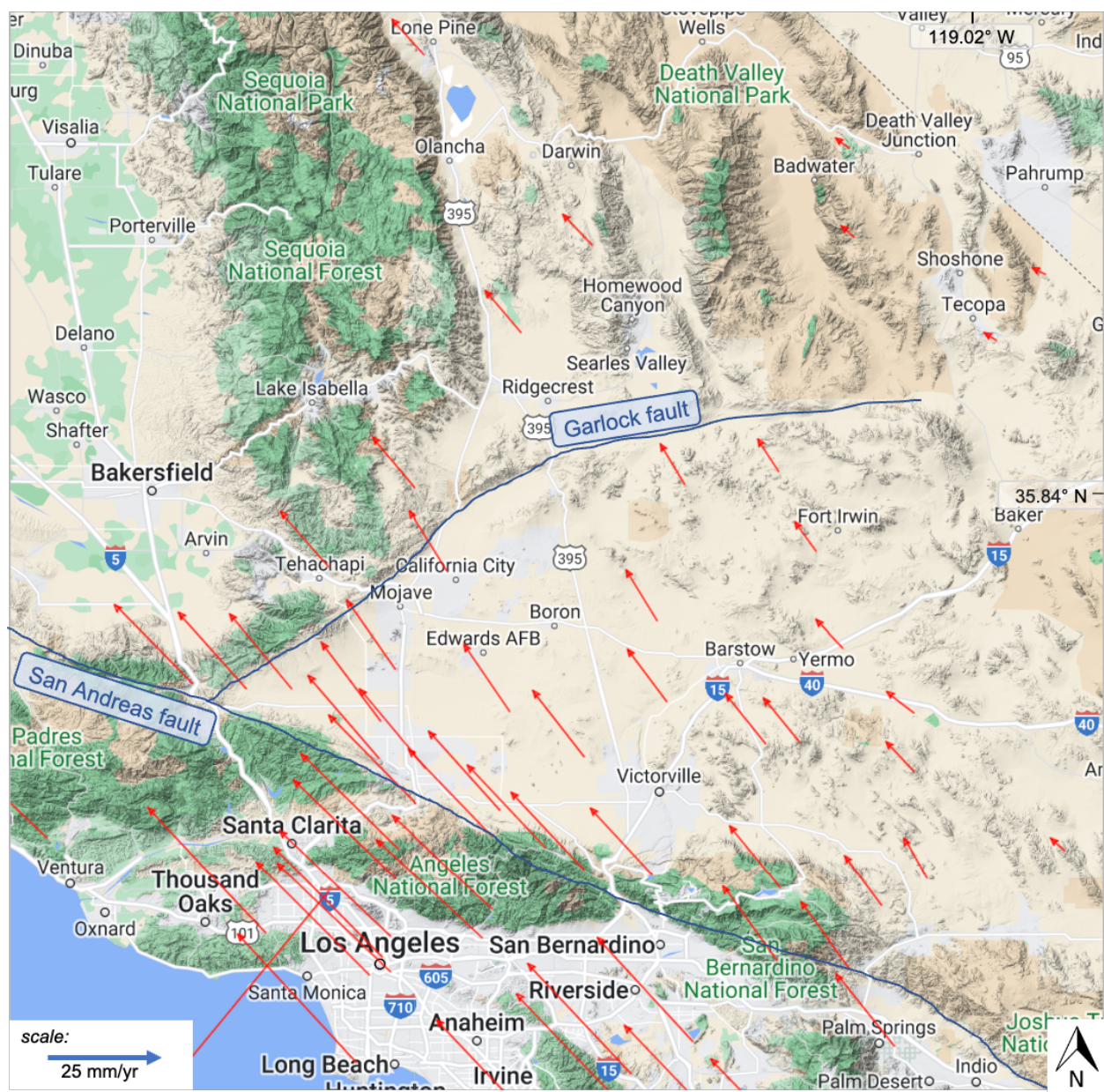
Figure 2-1. Global Positioning System (GPS) crustal velocity map of southeastern California around the regional tectonic regions. Data source is Global Navigation Satellite System (GNSS) N. America, NAM14, UNAVCO. Map created from EarthScope Consortium's Geodetic Facility for the Advancement of Geoscience (GAGE).
