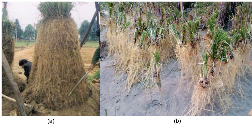
Fig. 4. (a) Length of Vetiver roots [reprinted from Kim et al. (2022), under Creative Commons-BY-4.0 license ( https://creativecommons.org/licenses/by/4.0/ )]; and (b) Vetiver roots grown in poorly graded sand for 110 days (reprinted with permission from Springer Nature: Springer, Innovative Infrastructure Solutions , “A simple approach for estimating contribution of vetiver roots in shear strength of a soil–root system,” F. F. Badhon, M. S. Islam, Md. A. Islam, and Md. Z. U. Arif, © 2021).
