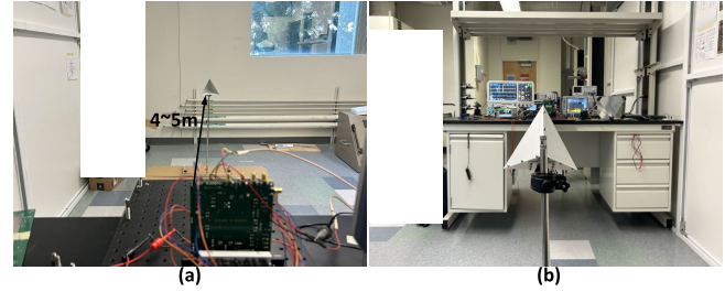
Fig. 37. Radar field measurement with corner reflector object. (a) Radar field measurement taken from the chip side. (b) Radar field measurement taken from the object side.
