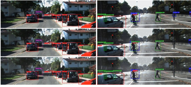
Fig. 6: Detection Performance of RAF-RCNN on Rainy KITTI Dataset under Various Rainfall Conditions (5mm, 25mm, 100mm)
