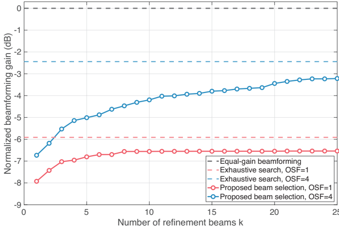
Fig. 4. This figure presents the beamforming gain provided by the selected top-k beams, compared to the equal-gain beamforming (upperbound) and the exhaustive search. The oversampled codebook is generated with the oversampling factors (OSFs) of four in azimuth and elevation dimensions.
