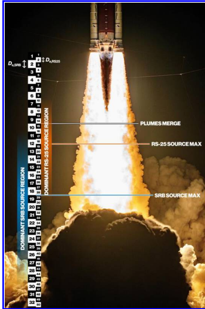
Figure 2. SLS's visible plume after the nozzle exit, with a marker indicating the beginning of the plume merging region. The rulers on the left indicate distance relative to the exit diameters of a single RS-25 and SRB, allowing for visualization of the dominant noise source region from 10\text{--}30 D_e downstream. Photograph by Josh Dinner from Space.com, used with permission.
