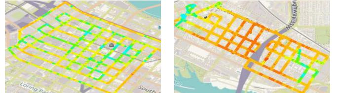
Fig. 3: Radio coverage maps for real RSS measurements. Green color represents strong RSS, while red poor RSS.
