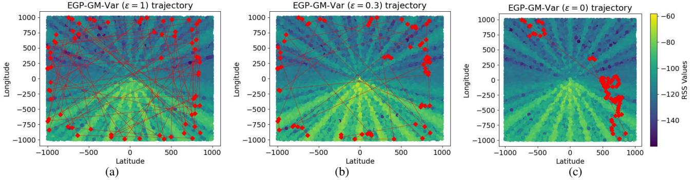
Fig. 11: Trajectory of the queried locations from the EGP-GM-Var method for (a)  $\varepsilon = 1$ ; (b)  $\varepsilon = 0.3$ ; and  $\varepsilon = 0$  in the high-band open space dataset.
