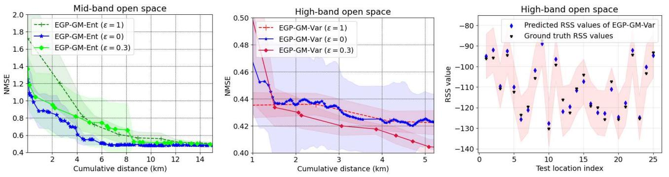
Fig. 12: NMSE vs cumulative distance of the EGP-GM-Ent method for different values of  $\varepsilon$  for (a) mid-band open space dataset; (b) high-band open space dataset; and (c) uncertainty quantification performance of EGP-GM-Var on the High-band open space dataset (RSS values are in dB).
