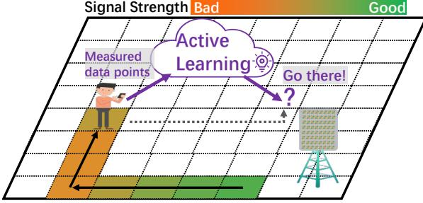
Fig. 1: Accelerating 5G Measurements via Active Learning.
