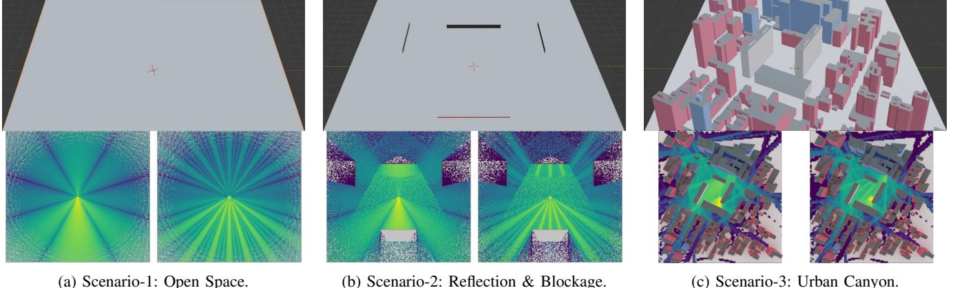
Fig. 2: Radio coverage maps of diverse scenarios rendered with Blender (top) and Sionna ray-tracing simulator at 3.7GHz (bottom left) and 26GHz (bottom right).
