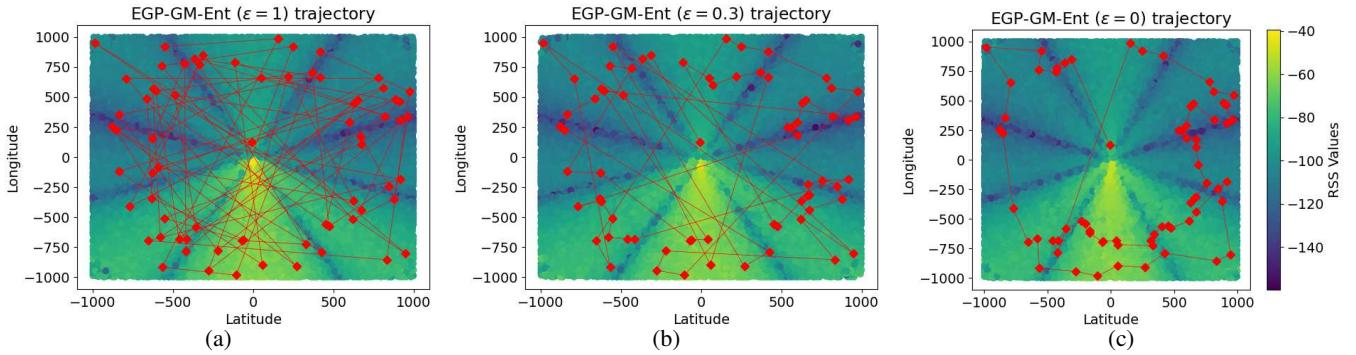
Fig. 10: Trajectory of the queried locations from the EGP-GM-Ent method for (a)  $\varepsilon = 1$ ; (b)  $\varepsilon = 0.3$ ; and  $\varepsilon = 0$  in the mid-band open space dataset.
