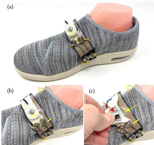
Figure 5: (a) The self-tightening shoe prototype incorporates an electromagnet for fastening. (b) the fastening system. The constriction of multiple SMA springs can pull the elastic band tight, forming the closure. (c) the electromagnetic latching mechanism. The red arrow indicates the electromagnet, while the yellow arrow indicates the passive magnet.
