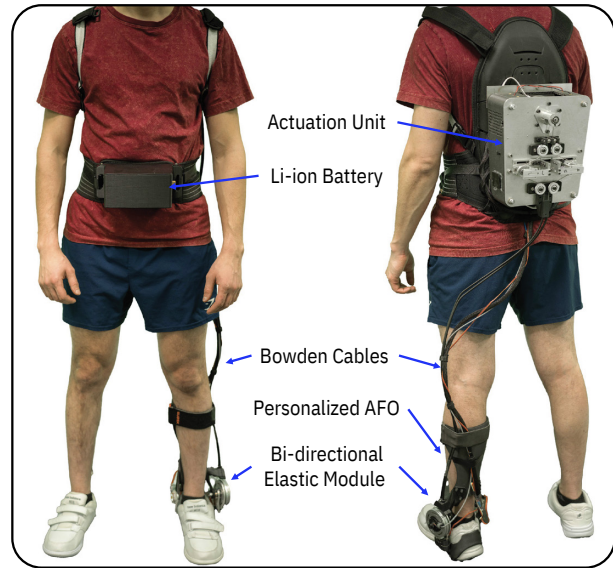
Fig. 1. Portable ankle exoskeleton Strider for gait training.
