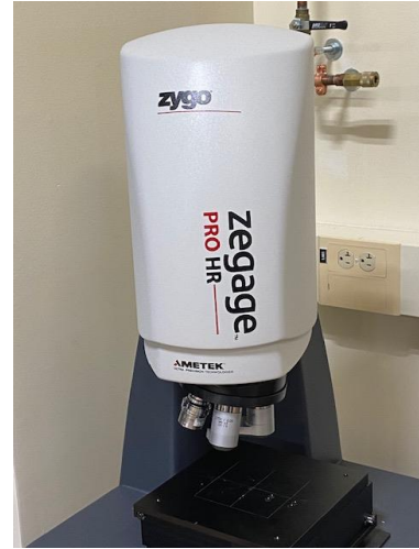
Figure 4: Zygo ZeGage used for measurement of the surface of the sample during the experiment.
