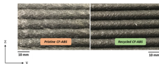
Fig. 2. Surface imaging is provided for the pristine (left) and recycled (right) printed parts.
