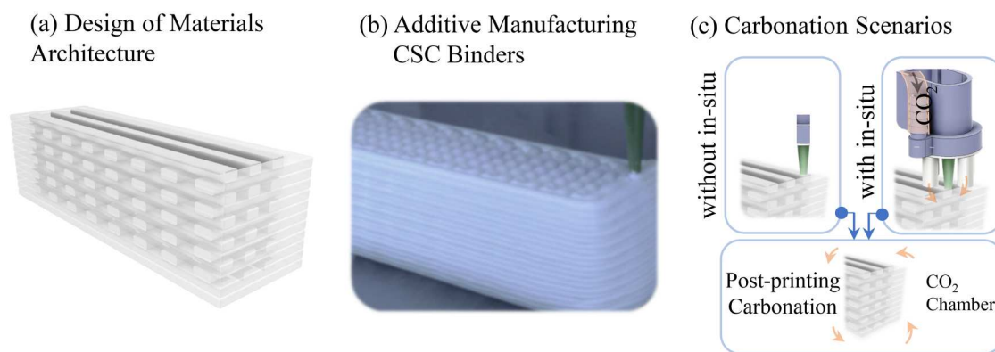
Figure 1. Three main approaches to enhance the carbonation and strength of CSC binders include (a) design of materials architecture, (b) additive manufacturing, and (c) two carbonation scenarios of without and with the in-situ carbonation using in-line \text{CO}_2 circulation nozzle, both followed by post-printing carbonation in a \text{CO}_2 chamber.
