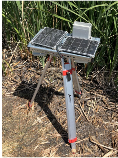
Figure 3. Deployed LEWIS 5 Sonar and LEWIS 5 rainfall attached to a tripod.
