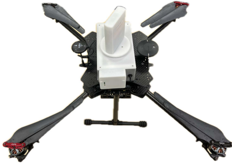
Fig. 1. Directional antenna with its 1-DOF rotating platform installed on a quadrotor UAV. The propeller blades are folded in the photo.
