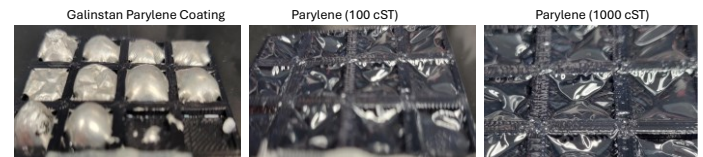
FIGURE 8: IMAGE OF PACKAGES AFTER 80°C SOAK TEST (18 DAYS).
