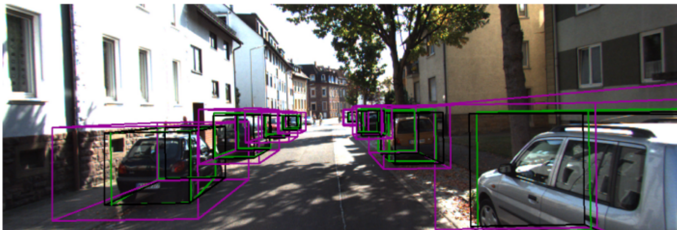
Fig. 4: Uncertainty in 3D Bounding Box Regression: Ground truth (black), predicted (green), and uncertainty (purple) 3D bounding boxes are visualized in a sample KITTI image of 8 cars with various occlusion and truncation status. As described in Section III-C, the uncertainty boxes represent a combination of upper- and lower-bound conditional quantiles obtained via conformal inference.
