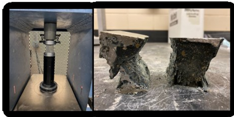
Figure 4. Test setup for 2-inch cube compressive strength.
