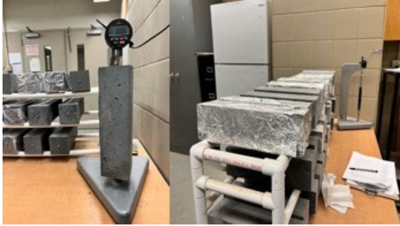
Figure 6. Drying and autogenous shrinkage samples (covered with aluminum foil to prevent moisture loss).
