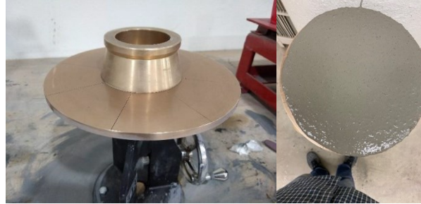
Figure 3. Measuring flow of fresh UHPC.
