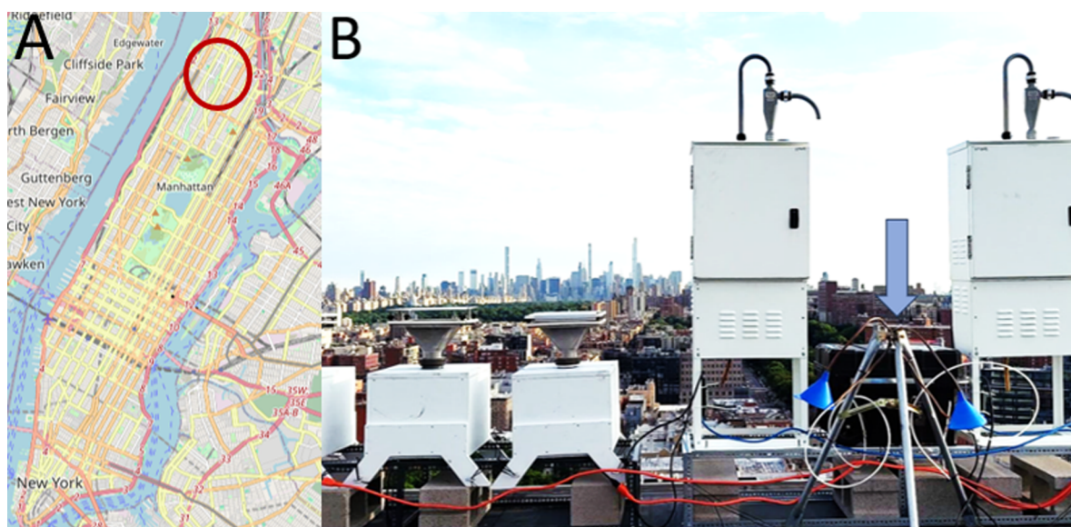
Figure 1. (A) Approximate location of sampling site in Manhattan, NYC. (B) Sampling equipment deployed on the roof of the ASRC. The samples described in this study were collected by low-volume samplers with the blue conical inlets in the right of the frame indicated by the blue arrow.
