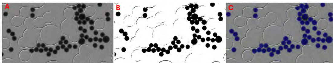
Figure 4.8: Circle Hough Transform Detection Method A) Background Subtraction and stabilization B) Adaptive Binarization C) Circle Hough Transform Detection
