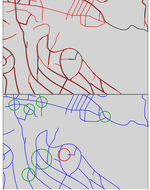
Figure 10: The input roadmaps OSM and TA are shown in black and red, respectively. The blue roadmap is the output. Green circles highlight successes, red circles indicate shortcomings.
