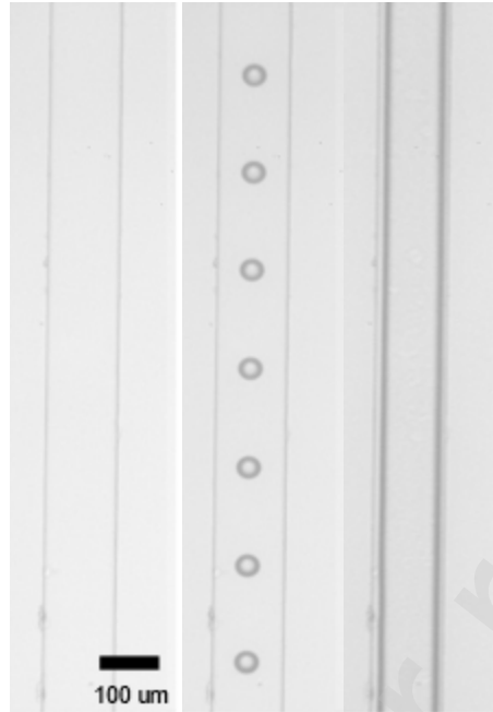
Figure 2. Representative training three flow regimes for CNN: (a) A liquid-dominated flow regime without bubble generation, (b) bubble generation in the dripping regime, and (c) air-dominated jetting regime.
