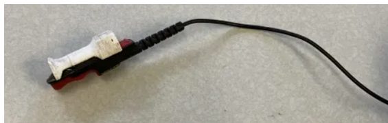
Fig. 14. contact microphone completed with 3D printed attachment.
