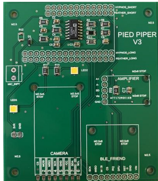
Fig. 7. The Pied Piper PCB after SMD components have been soldered.
