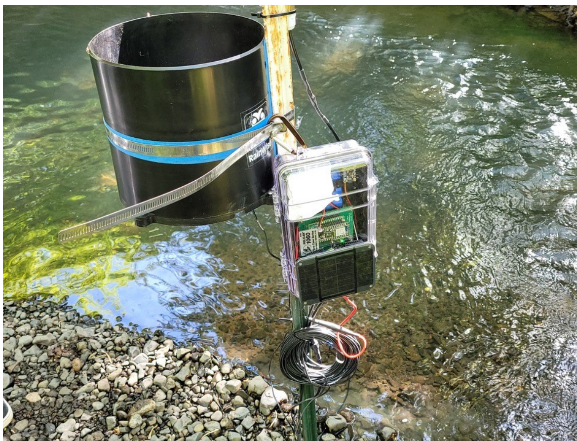
Figure 18. This figure shows a field-deployed WeatherChimes device.
