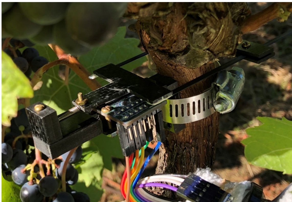
Figure 19. This figure shows a field-deployed dendrometer device monitoring the diameter of a grape vine to determine the amount of water being absorbed by the plant.
