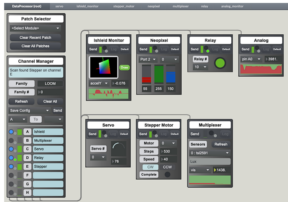
Figure 15. Max interface shows Wi-Fi connection client with real-time interactive sensor and actuator modules.
