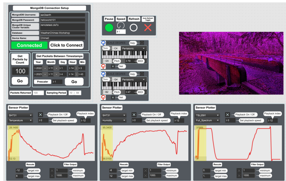
Figure 16. Max interface showing MongoDB database connection client, data plotter, data playback, sonification, and visualization module example. After connecting to the database, the user can parse individual data streams to plot over a defined time span and use those to shape audio signals and visual effects.
