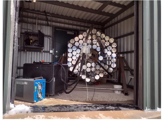
Fig. 16. The Trinity Demonstrator. In the front left is the Chiller for the cooling of the camera. Behind it is the crate with the readout electronics. The reflection of the camera can be seen in the mirrors of the Demonstrator.
