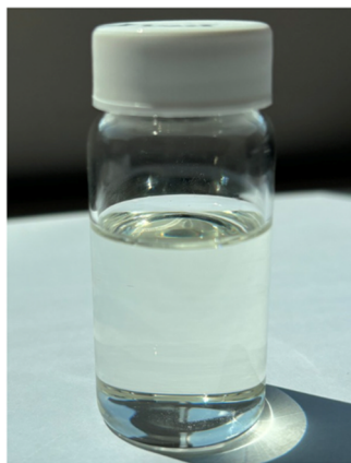
Figure 3. Colorless propyl 3,4,5-tris((2-ethylhexyl)oxy)benzoate, 3 , obtained after purification by column chromatography followed by Kugelrohr distillation and stored at room temperature, 23.5 °C, in air in the organic chemistry lab for 6 months.
