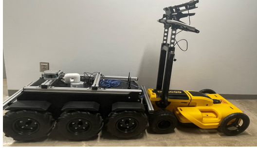
Fig. 2: Omnidirectional robot for GPR data collection, where the robot (HK1500) tows \varepsilon
