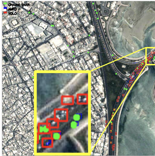
Fig. 3: Object detection results (human labels in green; YOLOv5 trained on DOTA in red; AMFD in blue). Yellow bounding box demonstrates domain shift issue of the model trained on DOTA and deployed on VISO.
