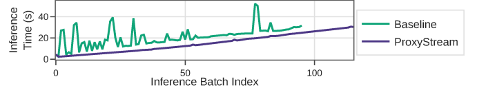
Fig. 9. Comparison of inference round-trip time between two DeepDriveMD implementations: baseline and ProxyStream. The size of each batch increases over time as the application accumulates more data points.
