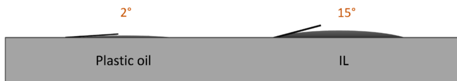
Fig. 5. Contact angle representation of PO and IL on steel surface after one minute duration.
